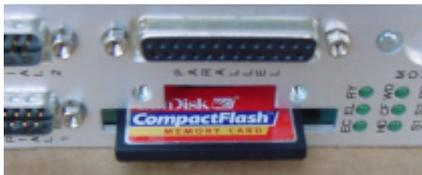
Illustration 43: partially pulled out CompactFlash card
