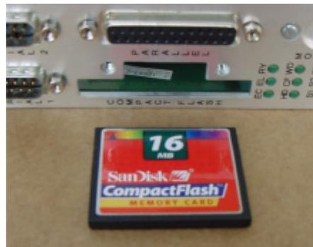
Illustration 42: removed CompactFlash card
