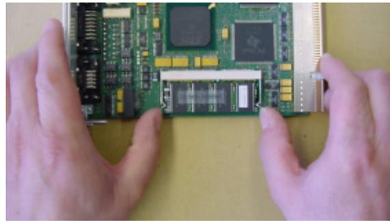
Illustration 48: removing the main memory module: pressing outwards the metal handles with the nails of the thumbs
