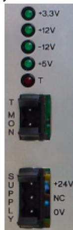
Illustration 25: OPS500 LEDs, temperature monitoring and 24V input
