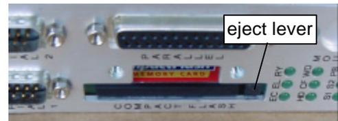
Illustration 40: CompactFlash slot without cover plate
