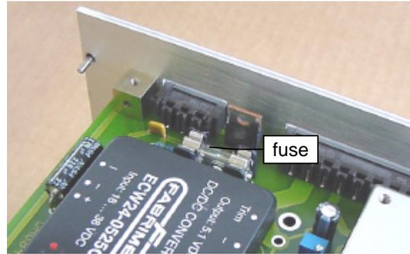
Illustration 28: exchangeable fuse of the OPM500 (variant 1)
