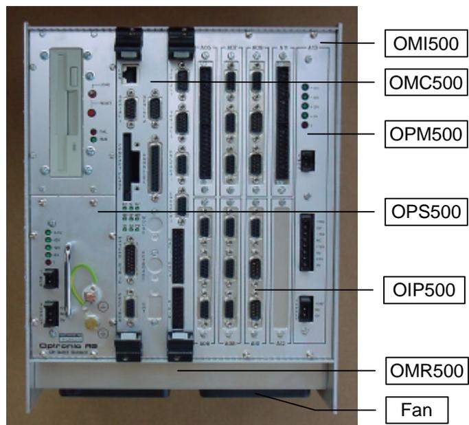
Illustration 2: „wide“ D500 with OMR500 (equipped with two fans), OPS500, OMC500, OMI500, OPM500, and seven OIP500
