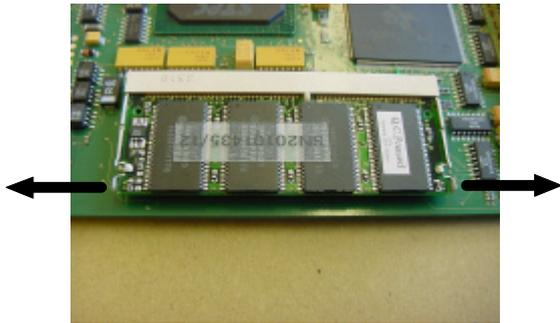
Illustration 47: removing the main memory module: both metal handles must be pressed outwards in direction of the arrows
