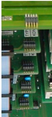
Illustration 65: add-on supply connectors of a OPM500 and four OIP500
