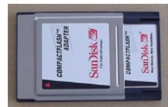
Illustration 37: CompactFlash to PC Card adapter with installed CompactFlash card
