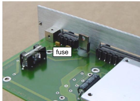
Illustration 26: exchangeable fuse of the OPM500 (variant 2)
