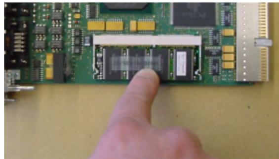
Illustration 50: inserting the main memory module: pressing the module into the retainer by use of the forefinger
