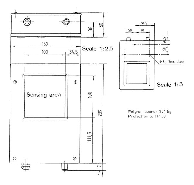
Sensitivity levels: 1mm - 2 mm - 4 mm - 8 mm - 16 mm The selected value is for a sphere of this diameter to be detected by the screen.
