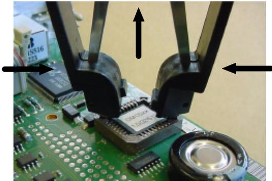
Illustration 51: operating the PLCC removing tool
