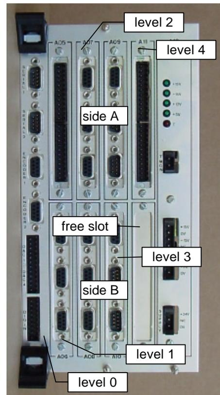
Illustration 57: exterior view „wide“ OMI500 equipped with seven OIP500 and one OPM500
