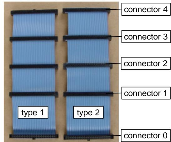
Illustration 61: two bus cables with five connectors for four OIP500s
