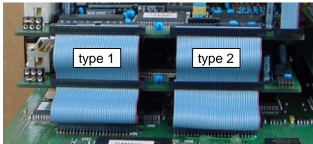
Illustration 60: bus cables attached at the OMI500
