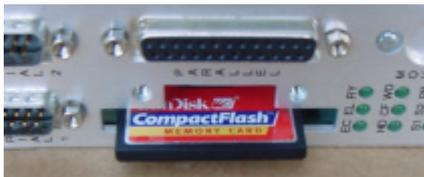
Illustration 43: partially pulled out CompactFlash card
