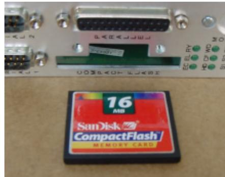
Illustration 42: removed CompactFlash card
