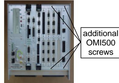
Illustration 13: OMC500 and OMI500 installed in a wide OMR500
