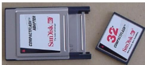
Illustration 38: CompactFlash card and CompactFlash to PC Card adapter
