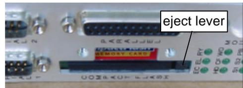
Illustration 40: CompactFlash slot without cover plate
