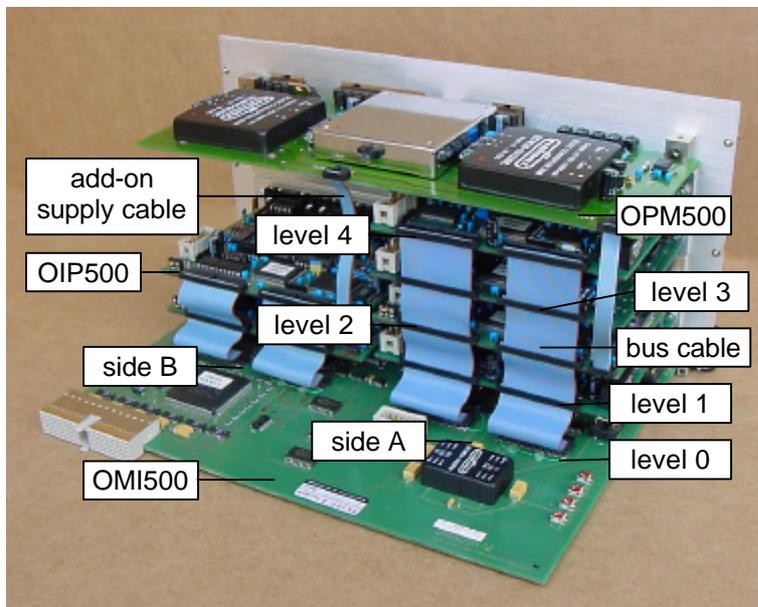
Illustration 56: interior view „wide“ OMI500 equipped with six OIP500 and one OPM500
