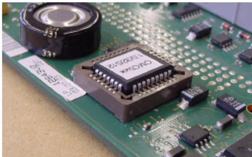
Illustration 54: inserting a new BIOS IC
