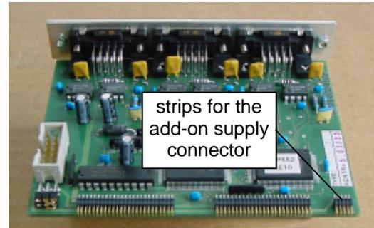
Illustration 66: OIP500 with strips for the add-on supply connector
