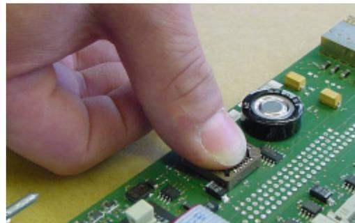
Illustration 53: press the BIOS IC into the socket
