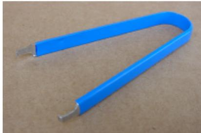
Illustration 68: special gripper for pulling out a connector
