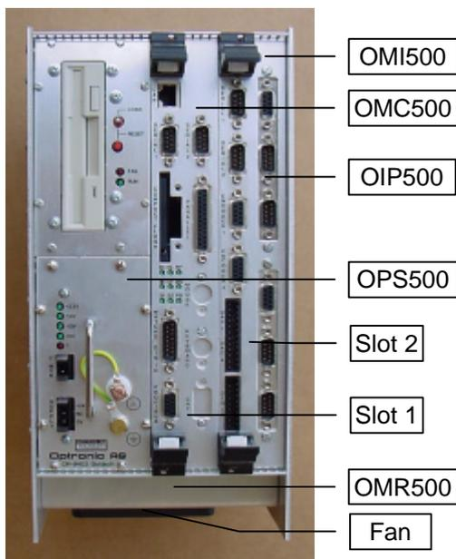
Illustration 1: „narrow“ D500 with OMR500 (equipped with one fan), OPS500, OMC500, OMI500, and two OIP500
