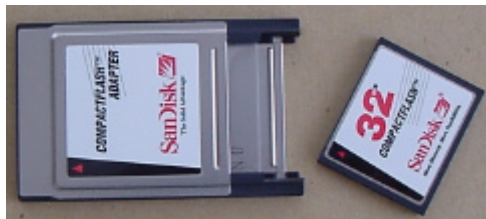
Illustration 5: CompactFlash Card and CompactFlash to PC Card Adapter
