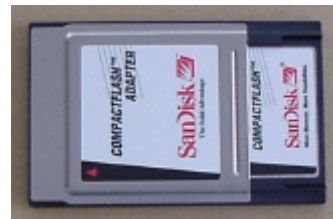
Illustration 6: CompactFlash to PC-Card Adapter with inserted CompactFlash Card
