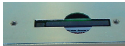
Illustration 4: CompactFlash Slot of an operating station with inserted CompactFlash Card and removed cover plate
