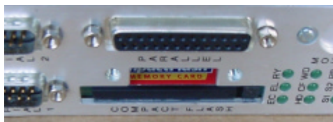
Illustration 3: D500 CompactFlash Slot with inserted CompactFlash Card and removed cover plate
