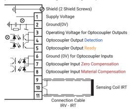
Output Detection: Conducting (condition ON): Material detected
